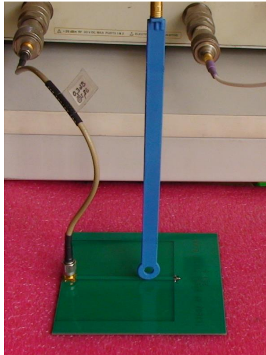
Picture 4 – measurement setup for coupling loss, 300kHz – 3GHz
