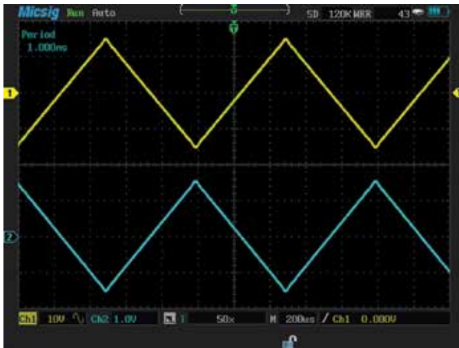
Fig.3: the 9-bit ADC means that the trace display is quite clean; much of the ‘fuzz’ visible here (such that there is) is due to the DAC producing the waveform, rather than the scope. The lack of signal linearity where the slope changes are quite clearly visible. It’s possible to zoom in on a section of the waveform by dragging a box using the touchscreen.
