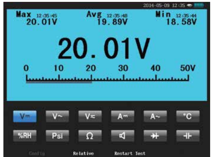
Fig.2: the unit operating as a multimeter, with the buttons to select various modes at the bottom of the screen. These can be selected using the touchscreen or side jog wheel. One soft button enables relative measurements while the other resets the statistics, displayed at the top of the screen. Time stamps for the min/max readings are a nice touch.
