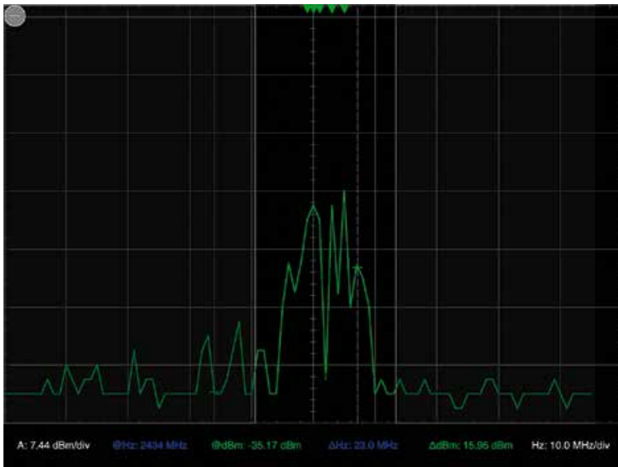
Fig.1: the WiPry in peak-hold/“decay” mode showing WiFi activity on channel 6. The grey masking on either side shows which frequencies are outside the currently selected channel although this can be hidden. Other modes such as Heat Map (shown in the lead photo) and Waterfall give a different display.
