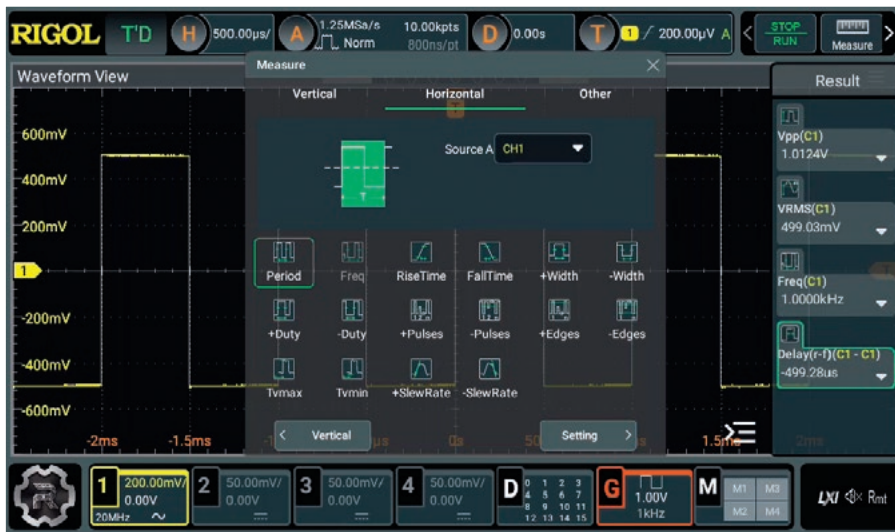
Screen 5: measurements are added to the Result panel at right. This panel can scroll up and down, so more than five results can be added. The options relating to the horizontal (time) axis are shown here.
