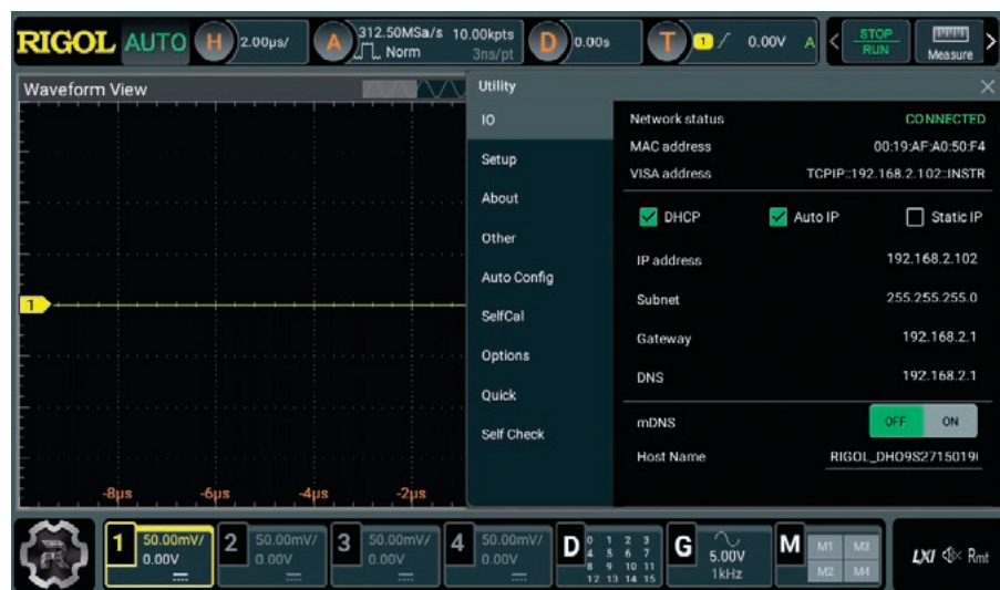
Screen 2: once we had the 'scope's IP address from this screen, it was easy to connect to the Web Control interface. The Utility menu also includes the setup and self-calibration options.
