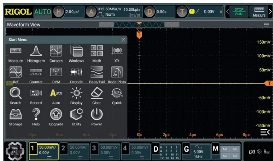
Screen 1: despite the numerous features, it's easy to find most menu options. A good place to explore is the R menu at the lower left corner of the screen. This also gives a good overview of the advanced features.
